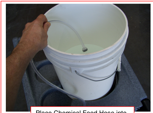
Place Chemical Feed Hose into Rinse Solution
