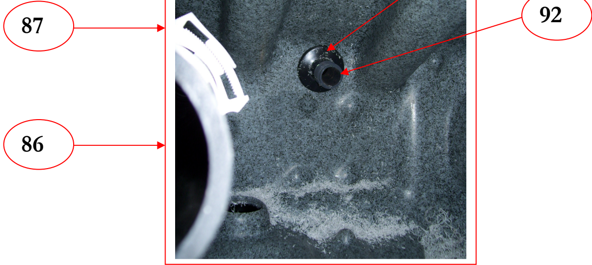
INSIDE RECOVERY TANK WITH OPTIONAL PUMP-OUT FILTER IN PLACE
