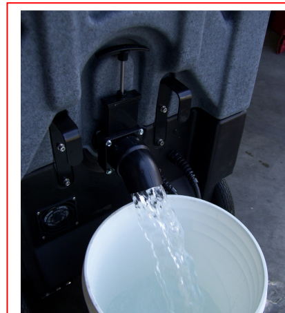
Drain water from Recovery Tank
