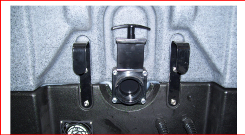
Remove four bolts holding valve assembly to flange fitting
